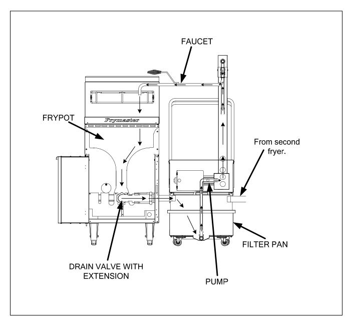
Arrows indicate direction of oil flow during the filtration process.
